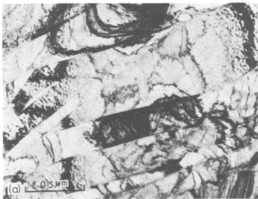
Figure 8 (a) Bright-field micrograph illustrating the microstructure of splat-cooled Er-80 at.% Zr alloy. (b) Dark-field micrograph corresponding to (a) showing precipitation within martensite platelets.
